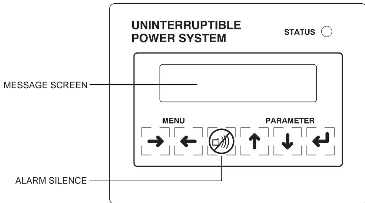
Figure 3-1. Digital Monitoring Panel
